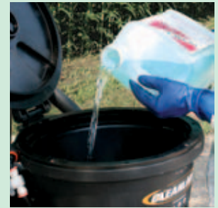
The Hypro Cleanload eliminates the need for operators to climb on and around machines while handling expensive and dangerous chemicals.
