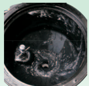
CycloRinse™ system provides premium cleaning and meltdown of flowable powders, such as AMS, with lid open for continuous-fill operation.
