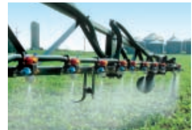
ULD tips (bottom) reduce drift significantly when compared to other nozzles on the market (top).
