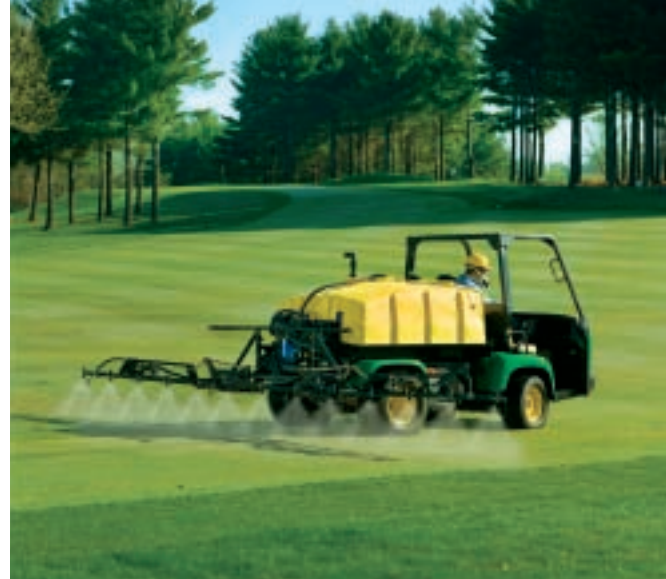
Drift reduction and coverage are two reasons ULD tips are standard on many golf course sprayers.
