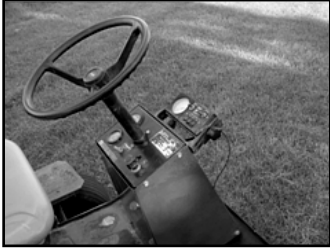
Monitors and controls were updated and moved offset to the driver's right to avoid having to reach around the steering wheel.
