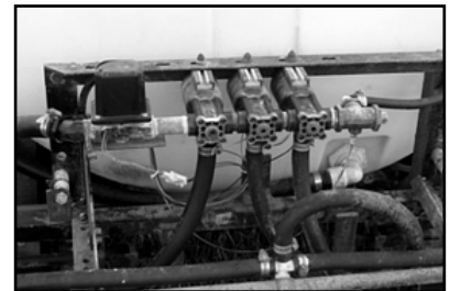
Simple on-off solenoids (above) were replaced with motorized plunger valves with a bypass feature (below).
