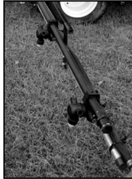
A wet-boom plumbing design cleaned up the look and removed a lot of worm-gear hose clamps.
