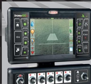
\* **SELETRON** must be connected to BRAVO400S computer since it allows the complete control of all boom and spraying functions. Thanks to the integrated GPS navigator, BRAVO 400S, through **SELETRON**, can control each and every stage of the spraying job individually: the only task the operator is left is to drive.
